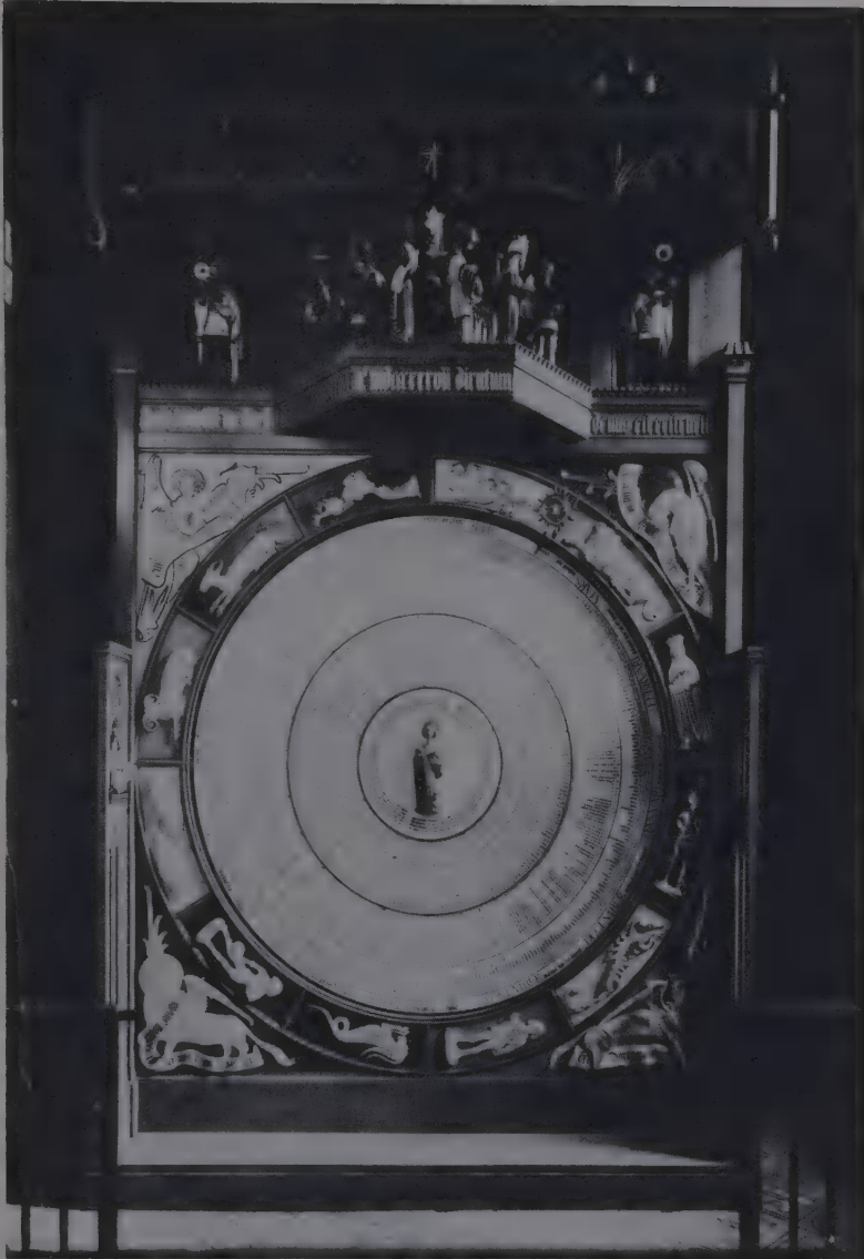
The face of the perpetual calendar; above it the Procession of the Wise Men. The great bell of the cathedral strikes the hour, when this ends a tiny organ within the clock plays an ancient plain song Christmas sequence, during which the procession of the wise men moves around the small platform
